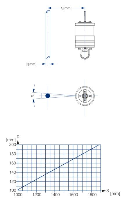
Diagram for choosing the minimum distance between obstacle and mounting plate.
