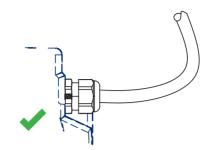
Include cable slack at the entering point of the cable gland
